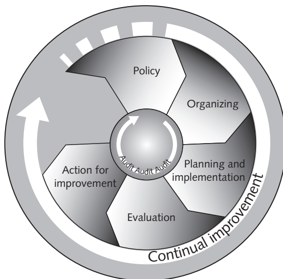
Figure 5.1 Main elements of the ILO-OSH management system (adapted from ILO, 2001).
